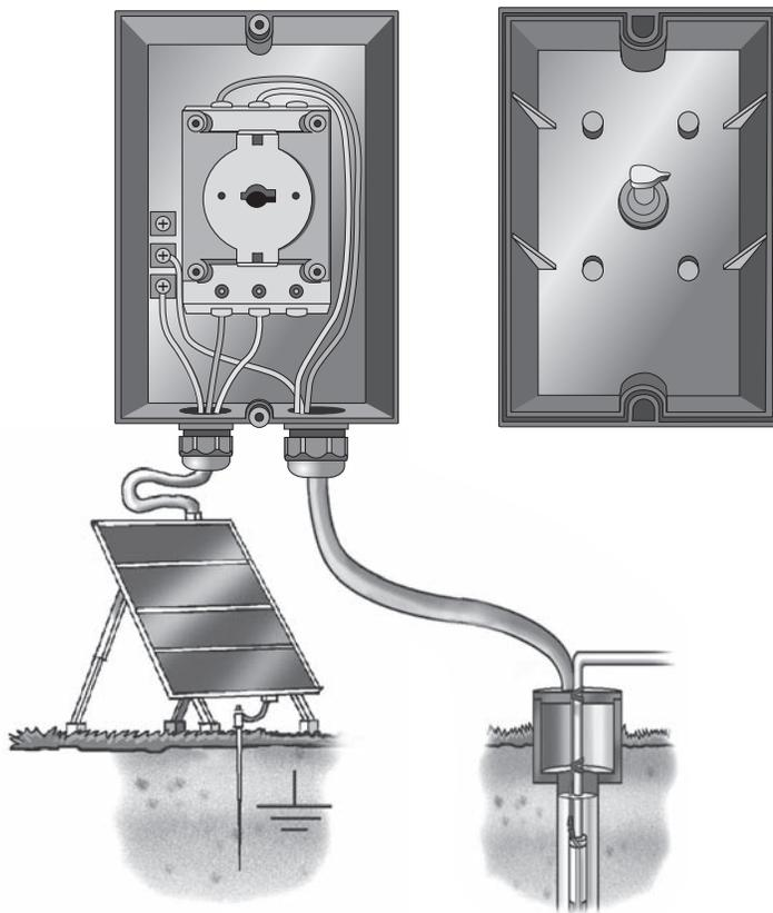
Internal (and external) wiring of IO 50 SQFlex switch box
