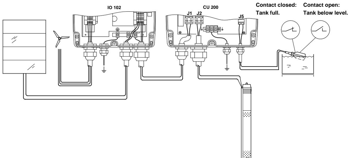
**Fig. 18.** Internal (and external) wiring for IO 102 SQFlex breaker box and CU 200 SQFlex control unit
