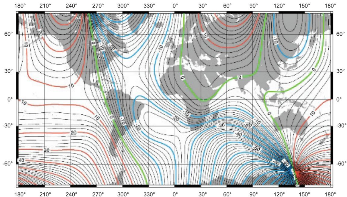
**Fig. 4.** The map illustrates the differences in magnetic declination in different parts of the world. Declination is caused by the fact that the geographic north pole and the magnetic north pole are not located in the same place. Depending on your location on the globe you must turn the solar modules away from the direction of the compass. How much appears from the map.
