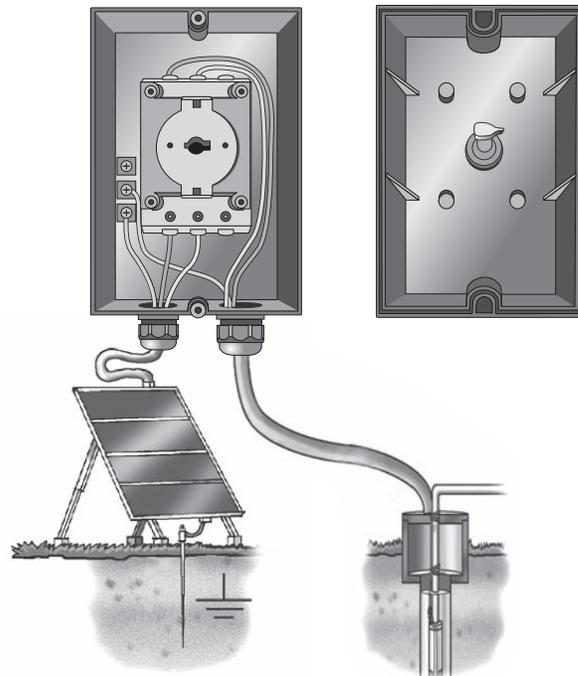
Fig. 6. Internal (and external) wiring of IO 50 SQFlex switch box.
