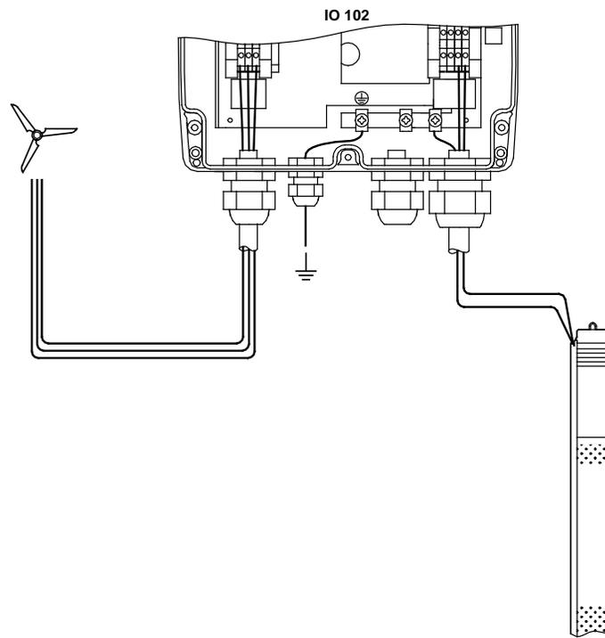
Fig. 12. Internal (and external) wiring of IO 102 SQFlex breaker box
